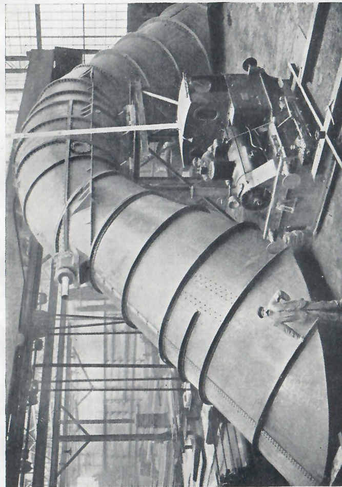
Fig. 14.—A Screw Pump for the "Electra" Pumping Works.
